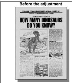
The background color of the original is also scanned. Therefore, no clear contrast is made between the background and image.
